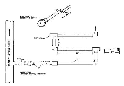
The Corrosion Rack illustrated here is a piping installation for water flow that is designed to be used for corrosion measurement. The right angle turns of this rack are designed to insert corrosion coupon holders. These holders ordinarily consist of steel or other threaded plugs with a Teflon® holder. To the end of this holder, a Corrosion Coupon is attached using a Teflon® screw and nut combination. A flow restricting orifice or flow rate indicator is used to simulate a critical flow rate.
